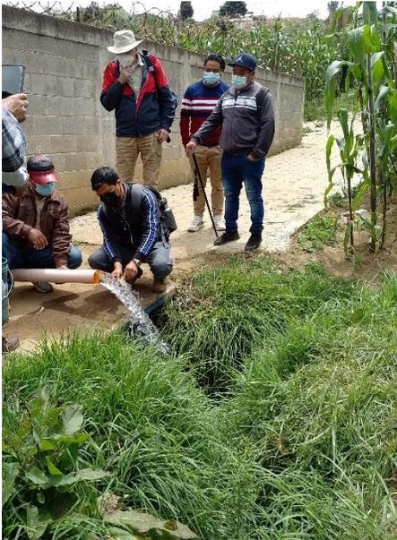
Well/pump flowrate measurement and water sampling
